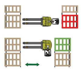
Standing to the side of the truck eliminates the risk of being trapped or crushed while allowing the Combi - PPT to operate in very narrow aisles.
